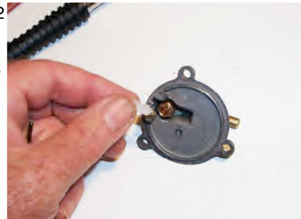
11. I like to install a new needle valve and seat every time I do a carb so it won't leak or flood.
