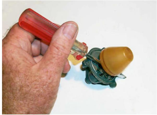
**14. The float needs to be set to close the needle valve at a specific height. On my H2 model the dimension was 5/16" which was the exact diameter of my screwdriver shank.**
