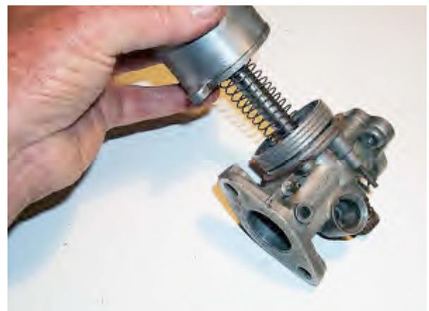
13. Put the piston and long damper spring in place, then, using a new gasket, attach the suction chamber housing.
