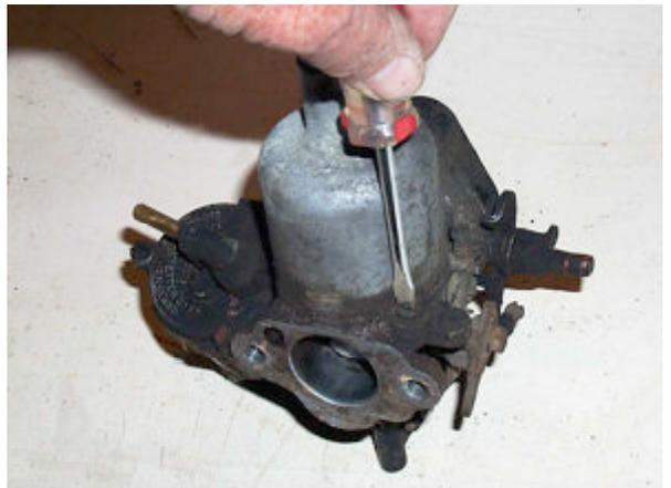
2. Remove the two screws holding the suction chamber body to the throttle body and lift it off.
