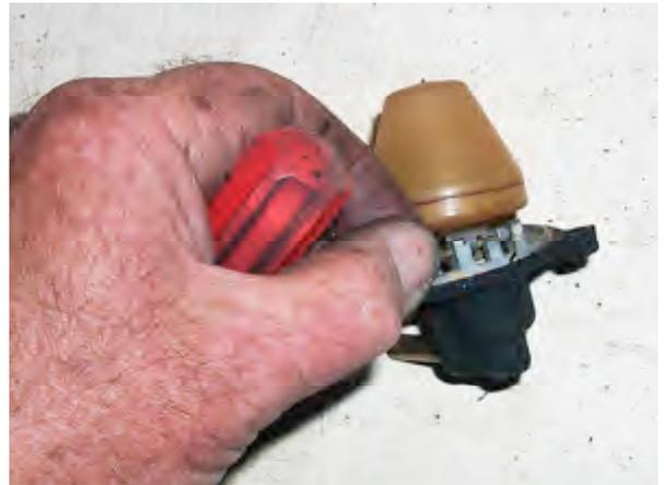
7. Remove the large bolt holding the float bowl onto the throttle body, then remove its top. Remove the float by pulling out its pin.
