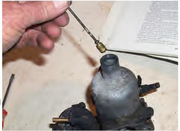
1. Begin disassembly by removing the piston damper assembly from the suction chamber body.
