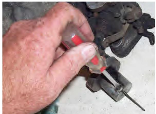
5. A flush mounted set screw holds the metering needle in place. Be careful not to cause any damage to the needle when removing it.
