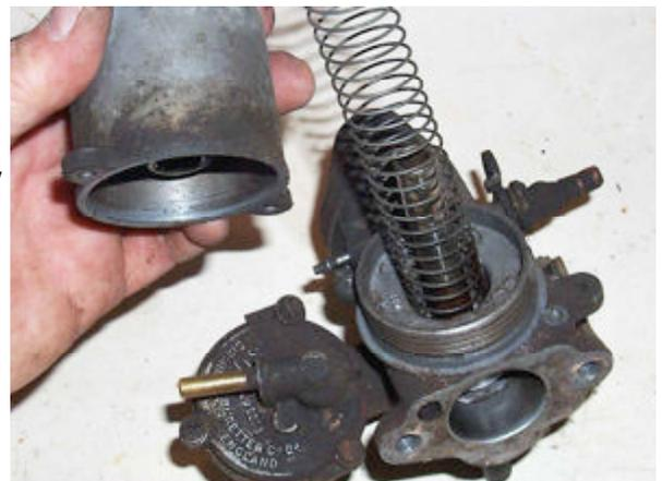
3. Under the suction chamber cover you'll find a long spring and the piston and needle assembly.
