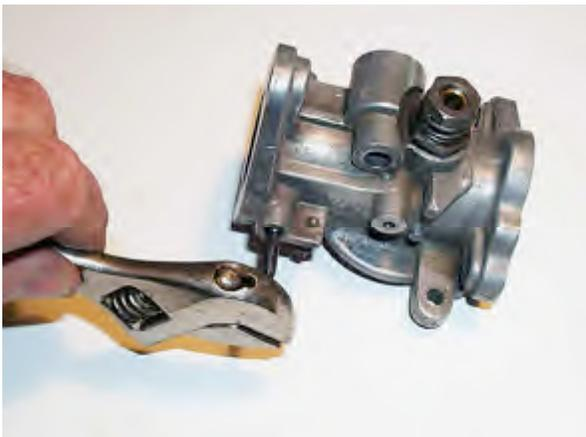
12. If you need to install a new over-size throttle valve spindle, ream the bearing surfaces to allow for a tight fit that permits the spindle to rotate freely.
