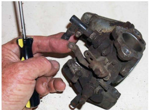
6. Disconnect the metal link to the jet assembly and gently push it aside.
