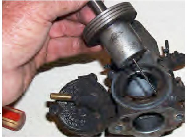
4. Lift out the suction chamber piston being careful not to knock or bend the metering needle out of center.
