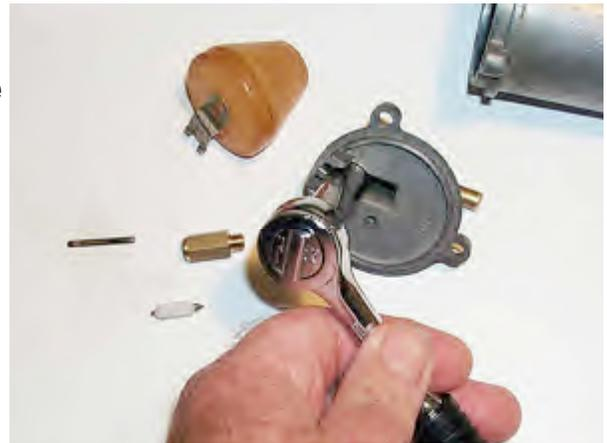
10. Lift out the needle valve and remove the old needle valve seat using a small socket.
